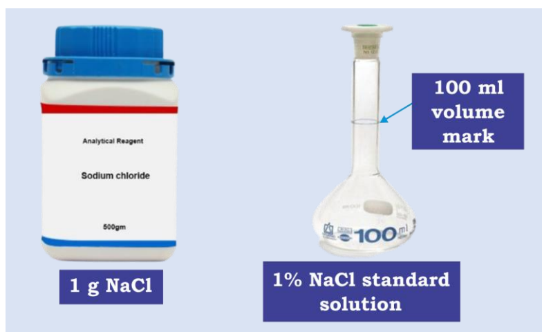
Fig. 2.5: Preparation of 1% NaCl standard solution.
